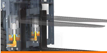
Buffering under the mast makes goods handling operation more comfortable;
