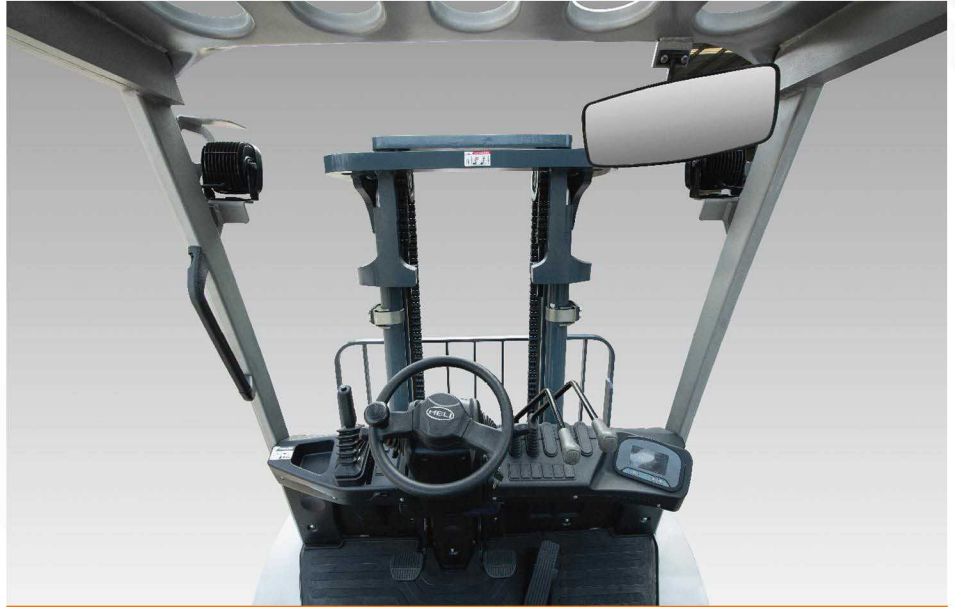
Wide view mast optimize the blind area of operation vision and it is comfortable and safe for operation;
