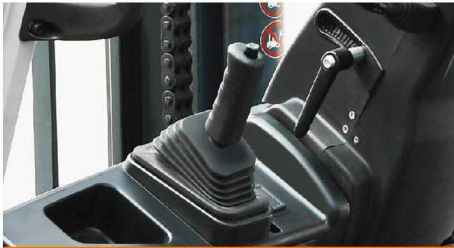
Ratchet type parking brake operating handle offers more labor-saving operation;
