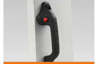
The armrest is equipped with horn switch for reversing.
