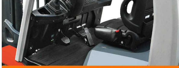
When the tilt cylinder sinks down in layout, the upper space of the bottom plate increases and the leg space is enlarged;
